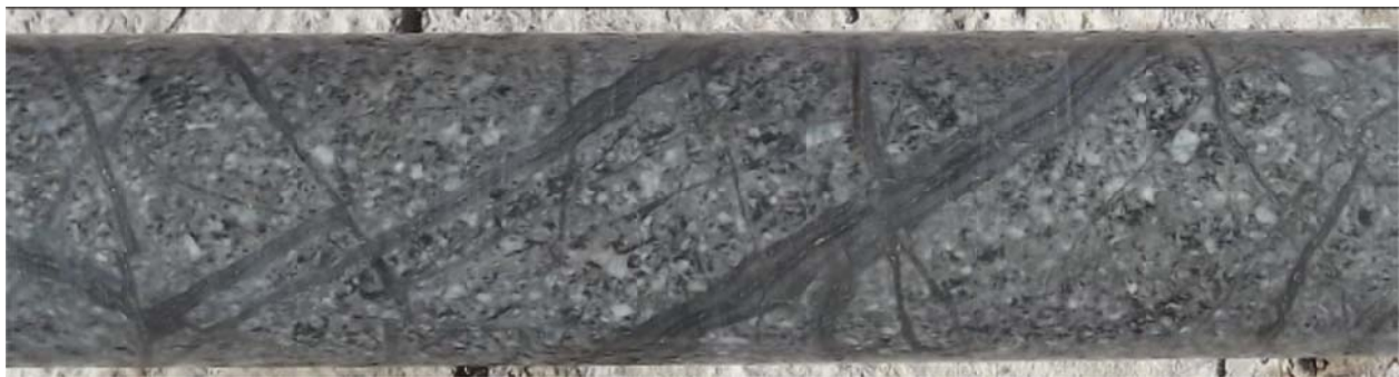
Figure 3: Drill core from RGR-12-100 at 624 m. Representative of a 3 m interval that contains 1.38 g/t Au and 0.299% Cu. Thin multidirectional banded gray veins are associated with gold-copper mineralization and contain quartz-magnetite-pyrite-minor chalcopyrite with a wall rock alteration assemblage of secondary biotite and potassium feldspar.
